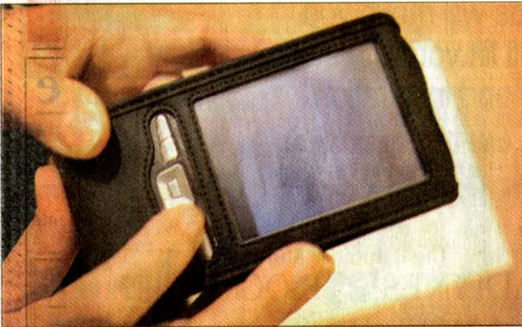
The 13-ounce Kurzweil-NFB Reader is a combination of a digital camera, a PDA and text recognition software that can convert a digital image of text into synthesized speech.
