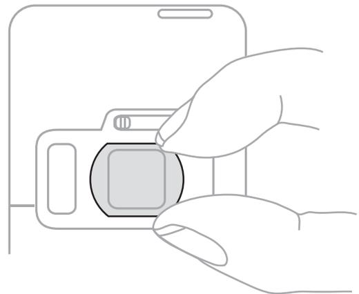
8. Hold the lens polarizer by the edges. Important: The flat edges of the polarizer should be **perfectly parallel** to the top and bottom edges of the camera assembly. Do not push on the center of the polarizer.
