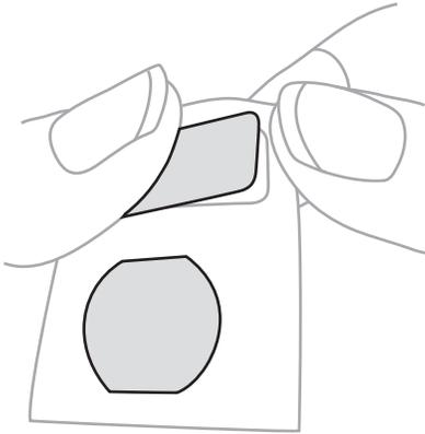
5. Grasp the flash polarizer between thumb and forefinger. With the other hand, bend the surrounding material down to separate the flash polarizer from the paper backing.
