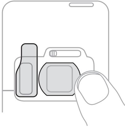
9. Push down around the edges of the lens polarizer that are touching the camera assembly. Do not push on the center.
