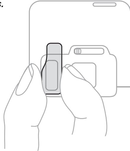
6. Hold the flash polarizer by the **edges**. Align the bottom left corner of the polarizer so it matches the bottom left corner of the silver metal around the flash. Apply gently, then nudge into place.
