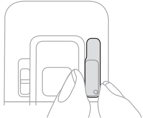
6. Hold the flash polarizer by the **edges**. Align the polarizer so the clear inner rectangle part of the polarizer covers as much of the flash window as possible. The flash polarizer should be placed just above the horizontal line across the middle of the phone. Apply gently, then nudge into place.
