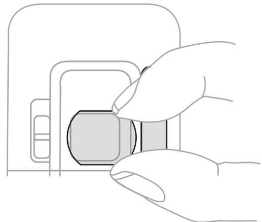
8. Hold the lens polarizer by the edges. Important: The flat edges of the polarizer should be **perfectly parallel** to the horizontal line across the middle of the phone, just under the lens in the figure. Place the lens polarizer close to the flash. Do not push on the center of the polarizer.
