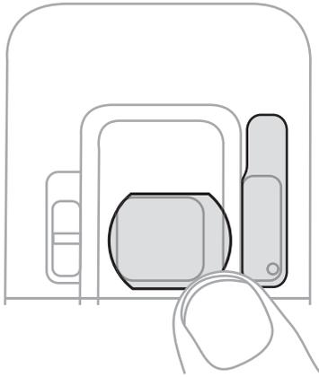
9. Push down around the edges of the lens polarizer that are touching the camera assembly. Do not push on the center.
