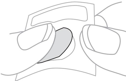
7. Bend the sheet so that the lens polarizer separates from the paper backing. **Do not bend the lens polarizer.**
