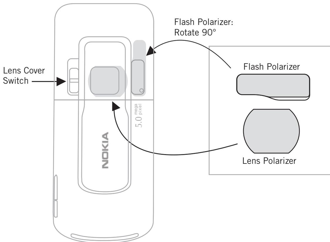
1. Open the lens cover with the lens cover switch (see figure above).
